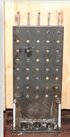
Seismic performance of CLT walls is governed by connections
