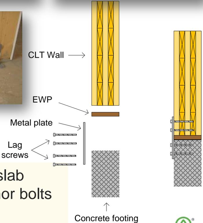
CLT wall to concrete wall or foundation slab using metal brackets or plates with anchor bolts & self tapping screws/lag bolts
