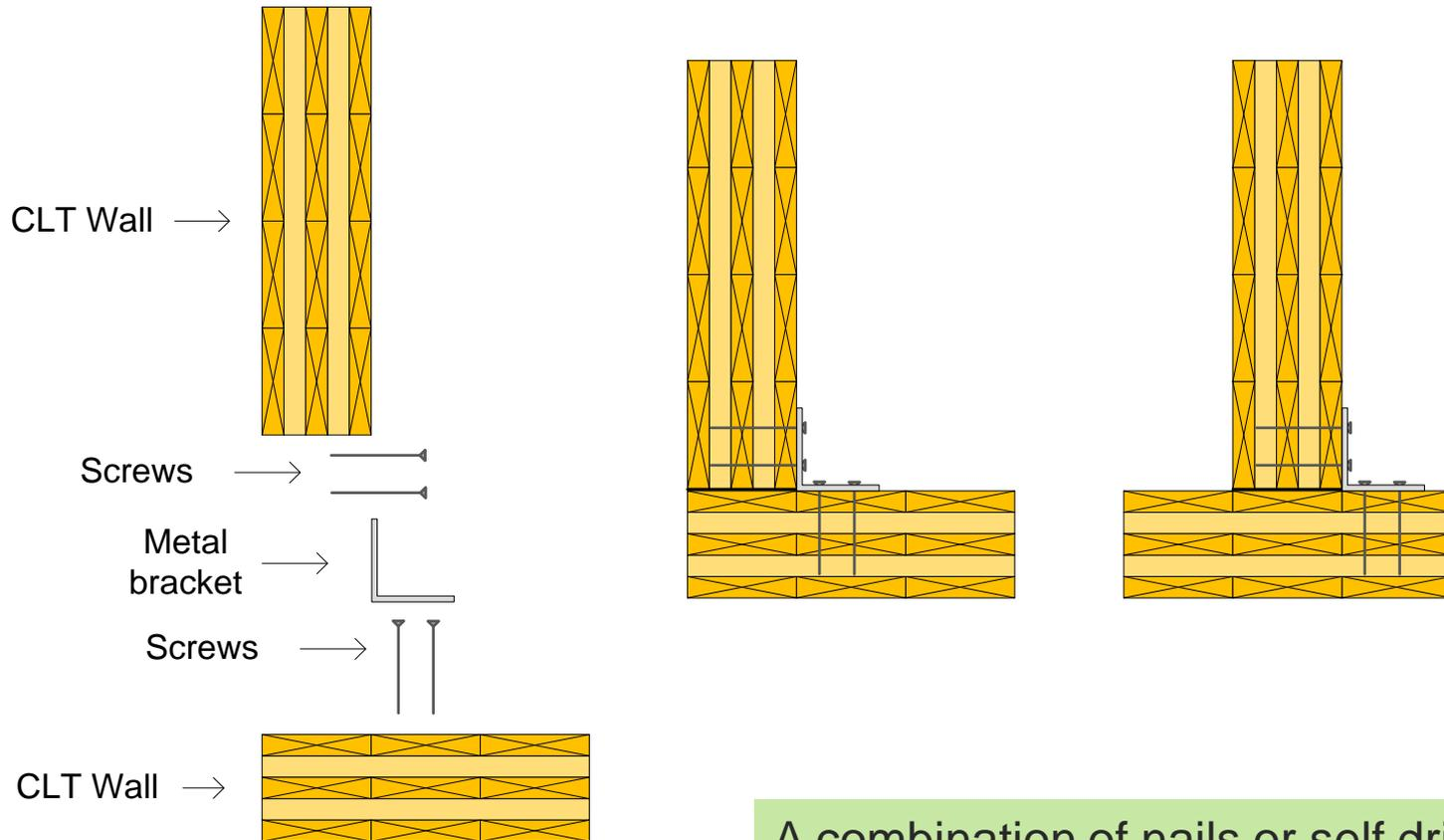
A combination of nails or self drilling screws and metal brackets
