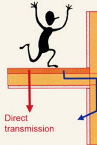
Surfaces of receiving room pass additional sound energy via structural vibration.
